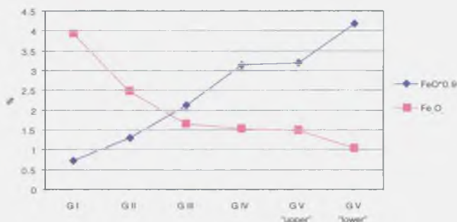
Figure 4. FeO → Fe 2 O 3 transformation during the weathering process
