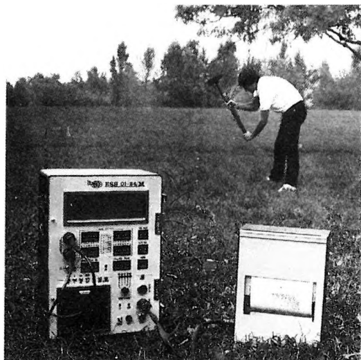
Field work with ELGI's 24-channel portable seismograph
