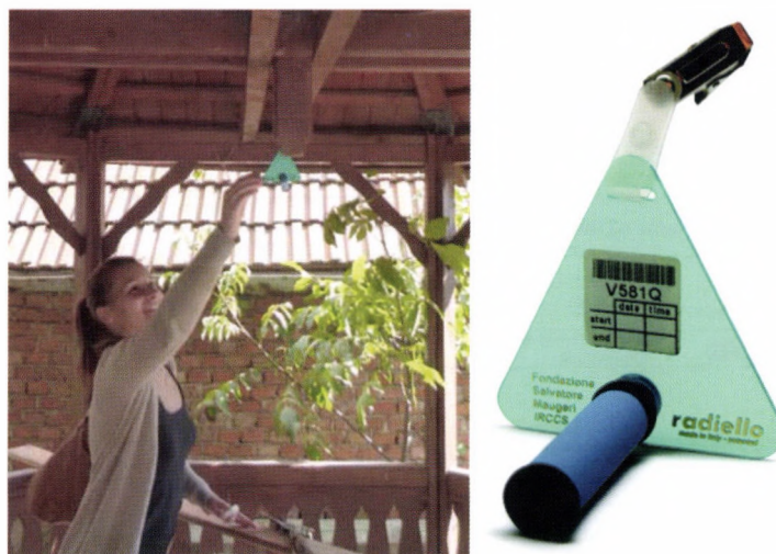
Figure 1. Radiello passive monitor probe and its allocation
