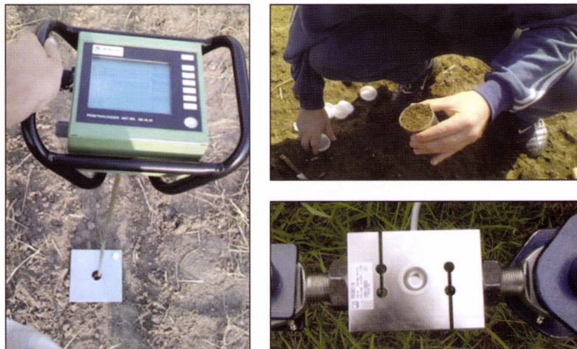
Figure 4. Eijkelkamp Penetrologger, soil sampling cylinders, load cell.
