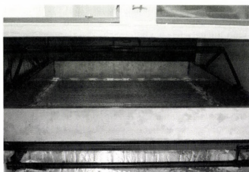
Figure 3. Shelf and heater of the experimental dryer
