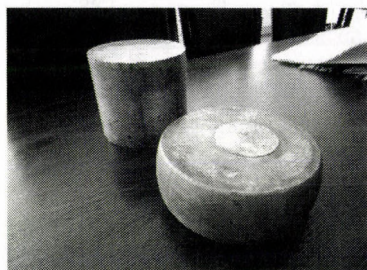
Figure 3. The original specimen (above left) and the forged specimen (bottom right)
