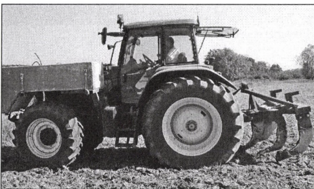
Figure 2 Tractor-subsoiler combination for the medium-deep loosening
