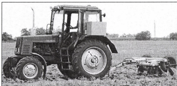
Figure 1 Measurement of soil electrical conductivity after medium-deep loosening [3]
