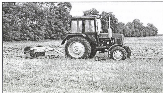
Figure 1 The measuring device Veris 3100 in a field-test on a loosened land
