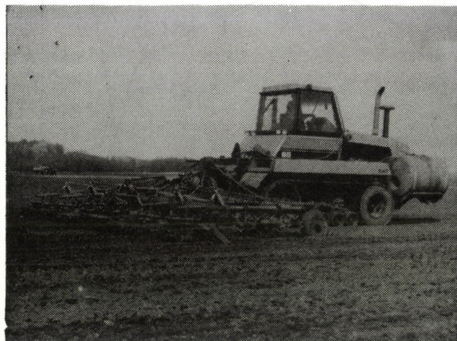
Fig. 4. Challenger-65 tractor with RAU-Unimat 8,4 seedbed preparator
