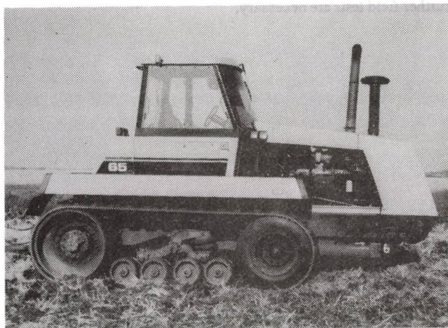
Fig. 1. Caterpillar Challenger-65 with rubber-belt track-drive.
