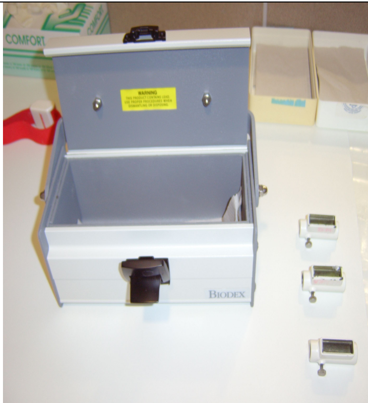
9. ábra: Ólomfalu kazetták Figure 9.: Containers made of lead
